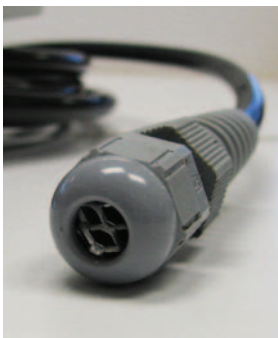
Above: Gutter sensor
