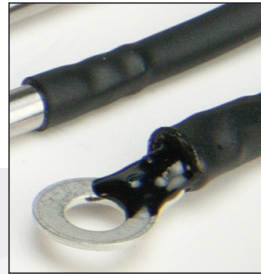
Above: Third channel remote probe
